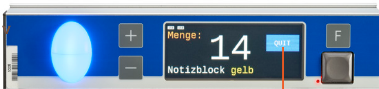
Resistive touch screen with freely definable softkeys (on-screen keys)
