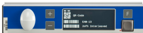
Resistive touch screen with freely definable softkeys (on-screen keys)
