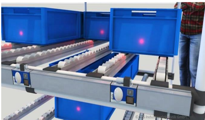
Level detection with TOF module and Put-to-Light compartment displays on the filling side of the flow rack [schematic illustration]
