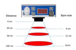
With few exceptions, the LED pointer option is possible for almost all PTF compartment displays. It thus supplements the classic eye-catching lamp by providing even clearer identification of the removal compartment.
