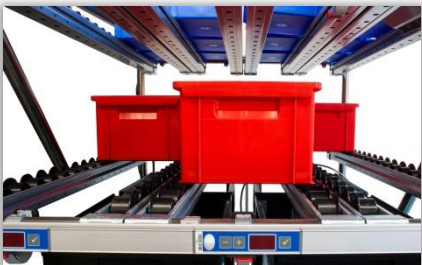
Level detection with E-Kanban module and Put-to-Light compartment displays on the filling side of the flow rack.
